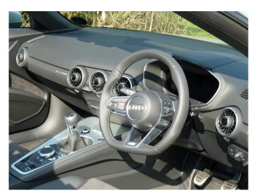
Modern dash design within a comfortable two seater cockpit. This car has a six speed manual gearbox. Note the 'drive select' rotatable control behind the gear lever.
