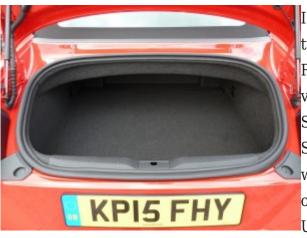
A practical feature is that the boot capacity is unaffected by the hood position; when open, the hood folds into its own tray above the luggage compartment.
