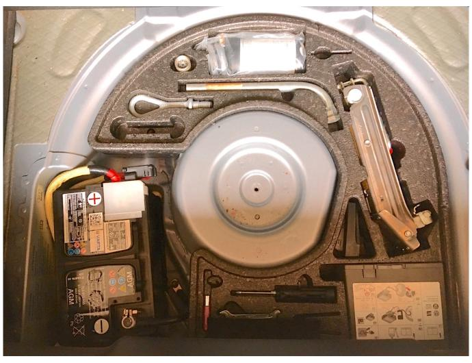
Reasonably complete and functional boot under-floor carries no-spare tyre repair system, some surviving tools and the relocated battery.
