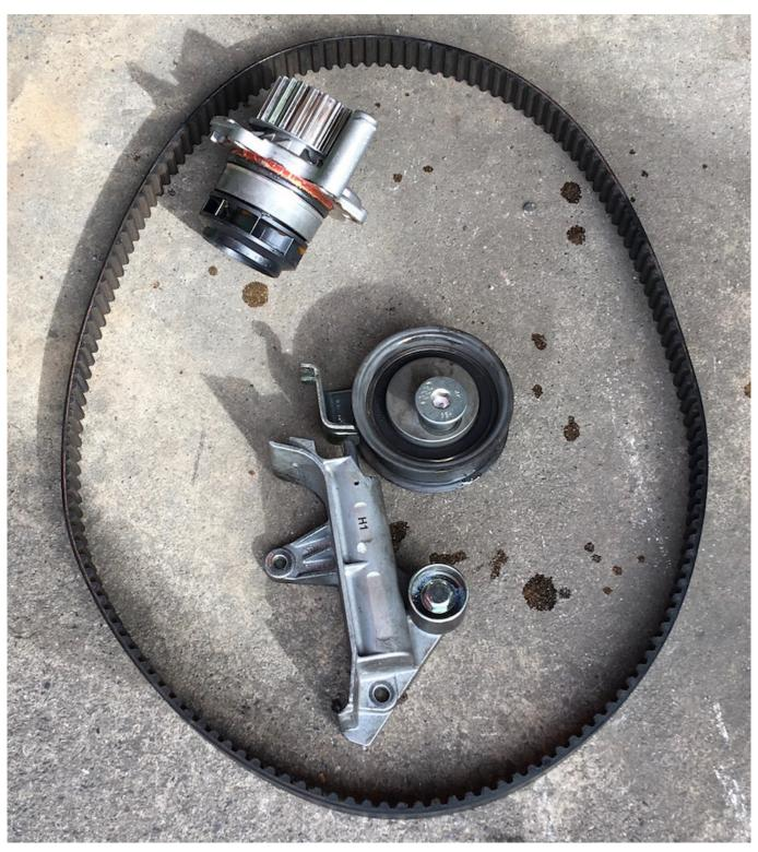
Finally decided that a specialist full service was necessary despite pre-delivery assurances: water pump renewed and cam belt was worn: worth a double check...
