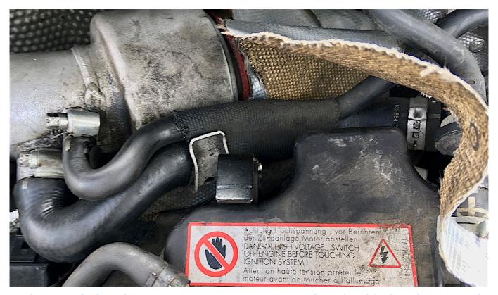
Split air intake breather pipe component cost £112 to replace, fitted for less than £50 and showed a perceptible improvement in part throttle turbocharger response.
