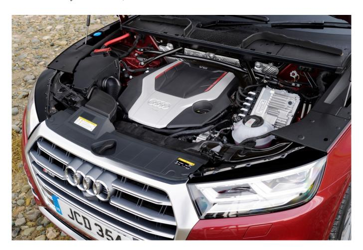
At the heart of the new SQ5 is of course the engine. The new 3.0 litre TFSI petrol unit is the successor to the unit first used by the S4 and S5 but the supercharger is replaced with a new twinscroll turbocharger located within the 90degree V of the cylinder banks. Not only does this engine supply 354 hp but also a huge 500 Nm (369 lb.ft) of torque available from
