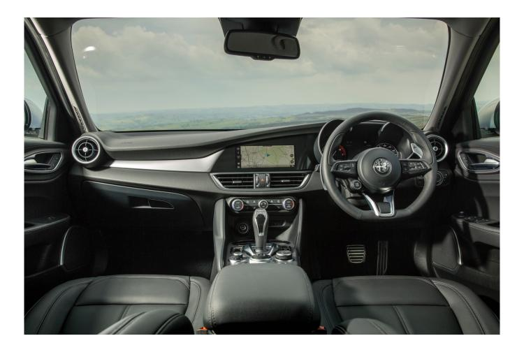
The central console provided a combination of touchscreen and remote operation and gave a variety of displays, some of which could be simultaneously shown for convenience. It was reasonably straightforward and always very clear.
