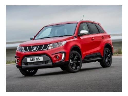
Move forward to the new 1.4 S turbocharged petrol version and this offers, 17% more power, 41% more torque and a 4% improvement in fuel economy over the naturally aspirated 1.6-litre petrol unit. It is just a pity that this engine is only offered in a new high S spec level.
